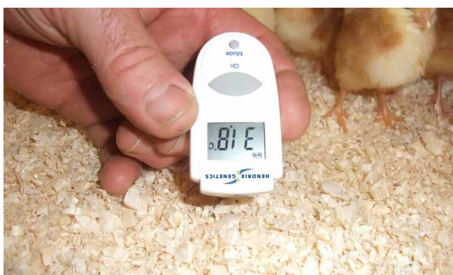
Measuring litter temperature
